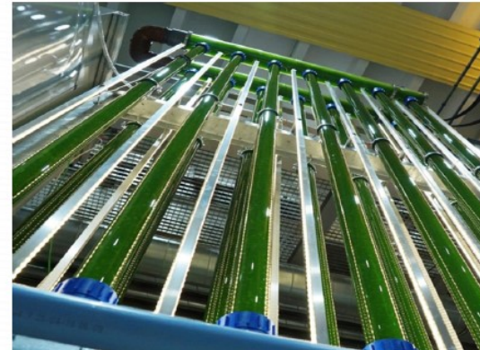
PBR artificially illuminated with a volume of 135 l, 3.5 m high, equipped with an airlift system for culture mixing
